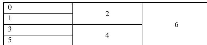
Figure 6: Wavelet Packet index pattern using EWPBTE. Numbers from 0 to 6 represent the enhanced indexing system. [13]
