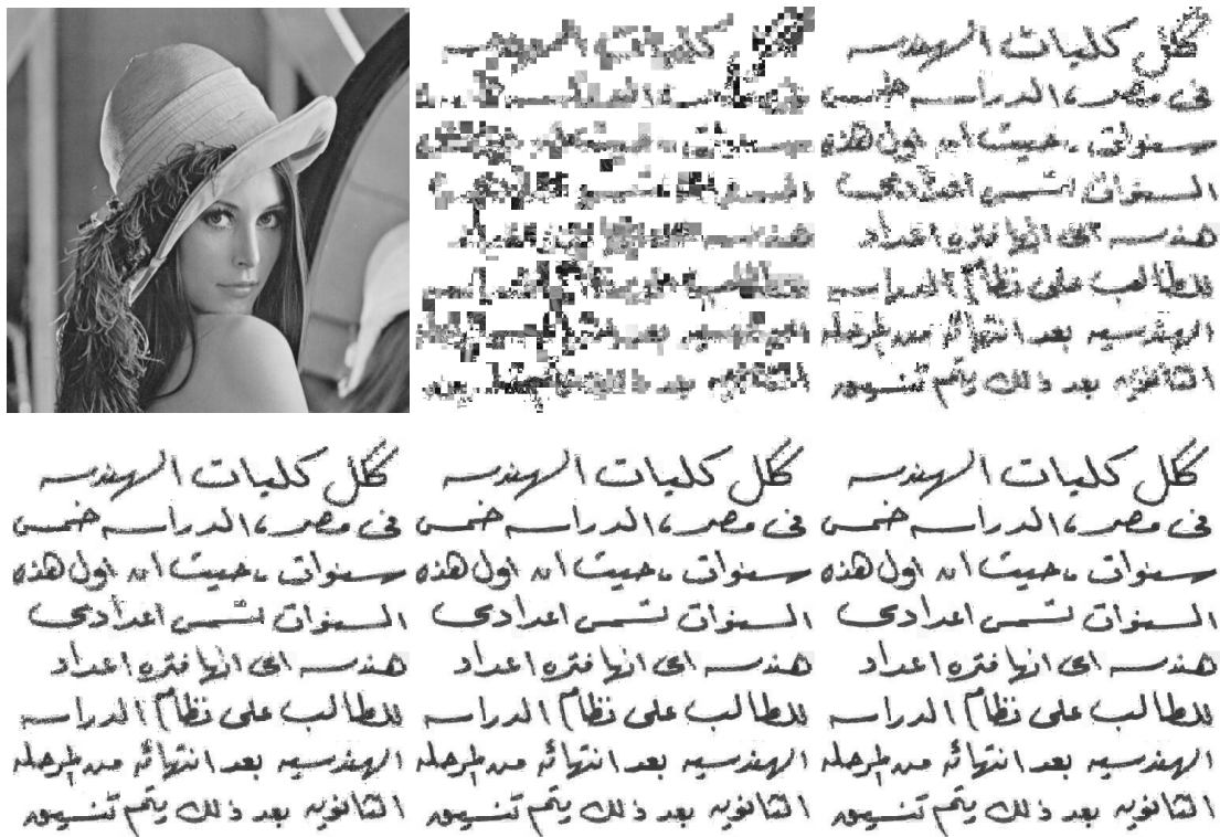
Figure 1: Iterations from the decoder, starting from an arbitrary image (left upper), converging to our document image (right down). Control parameter threshold =2
