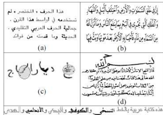
Figure 3. Illustration of a few characteristics of Arabic writing in the ARABASE database: : (a) Different sub-word of machine-printed text, (b) writing with diacritics, (c) free handwriting, (d) Historical handwritten documents, (e) multi-font machine-printed text, (Ben Amara, 2005).
