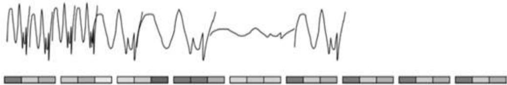
Figure 2: Speech signal is segmented into sequence of features frames.
