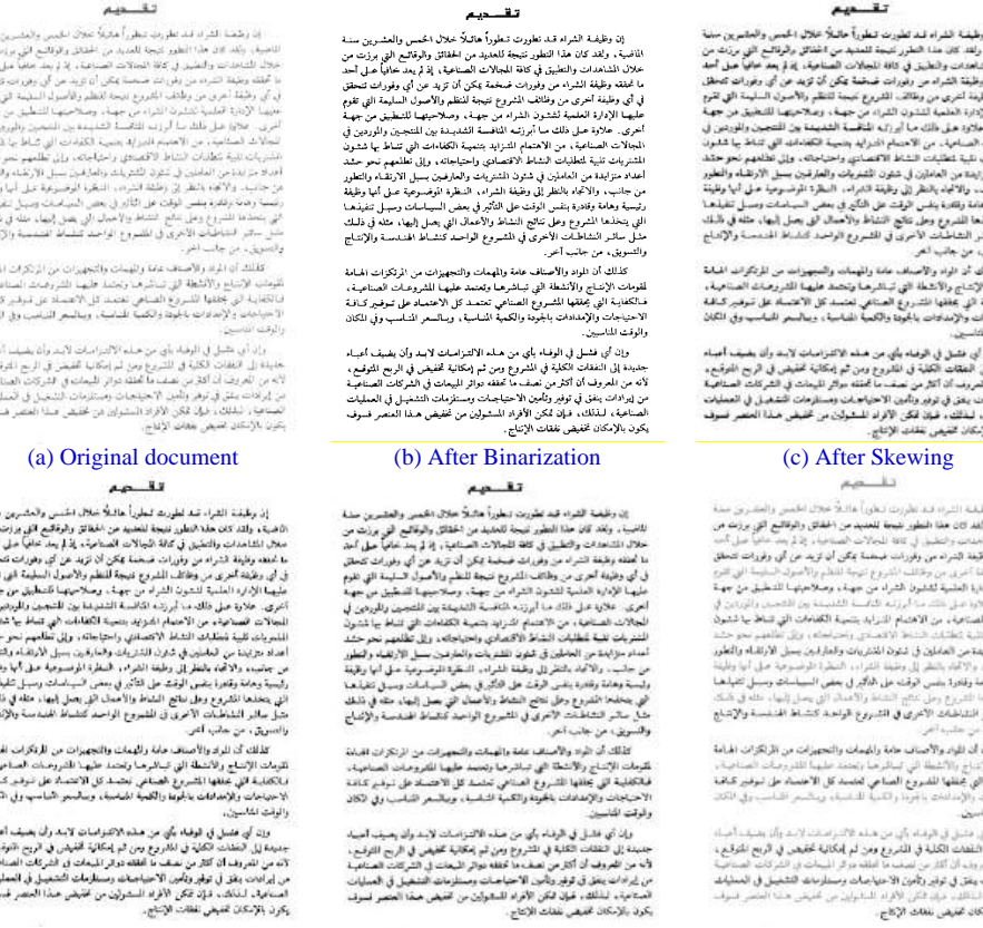
Figure 5: Example of Arabic document after the pre-processing processes
